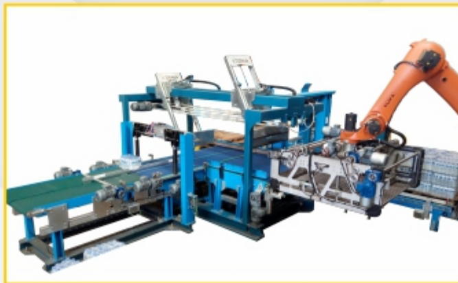
Complete Layer Robotic Palletizing (Can be used for any type of product.)
